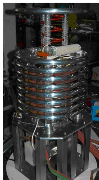
Figure 2: The 250-kV, 50-mA Cockcroft-Walton generator.
