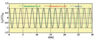
Figure 1: Simulation results ( $N_D=1,10$ ) and analytic solution  $\cos(k_y s)$  for no wake case with external focusing  $k_y=3$  m<sup>-1</sup>.
