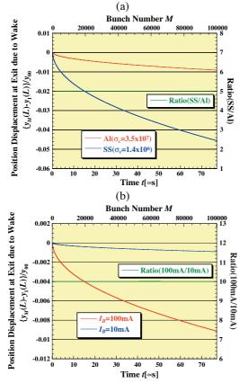
Figure 8: Position displacements at exit due to RW wake (a) for electric conductivities of pipes  $\sigma_c = 1.4 \times 10^6 \ \Omega^{-1} \ m^{-1}$ (SS: stainless steel) and  $3.5 \times 10^7 \ \Omega^{-1} \ m^{-1}$  (Al: aluminum) and (b) for the average currents  $I_B = 100 \ mA$  and 10 mA with all the Q-magnet on as a function of time. Their ratios are also shown.
