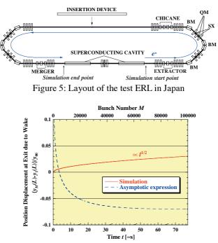
Figure 6: Position displacement at exit due to RW wake with all the Q-magnet off as a function of time and bunch number.
