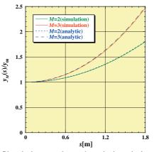
Figure 2: Simulation results and analytic solutions for the second and third bunches (M=2 and 3) in non-zero wake case ( $a=0.5 \text{ m}^{-1}$ ) without external focusing.
