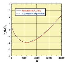
Figure 4: Simulation result ( $N_D$ =10) and asymptotic expression for strong focusing case (a=2.62x10<sup>-3</sup> m<sup>-1</sup>,  $k_y$ =3 m<sup>-1</sup>, L=10 m).
