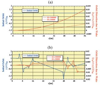
Figure 7: Initial orbits and orbit distortions due to the RW wake for M = 10000 and 100000 with all the Q-magnet (a) off and (b) on in the test ERL. The bunch numbers M = 10000 and 100000 correspond to the times t = 7.7 and 77 µs.
