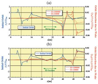
Figure 9: Initial orbits and orbit distortions due to the RW wake for M = 10000 and 100000 (t = 7.7 and 77 µs) with ID focusing strength (a)  $k_y = 0$  m<sup>-1</sup> and (b)  $k_y = 1$  m<sup>-1</sup> in a small-gap ID pipe at ID section.
