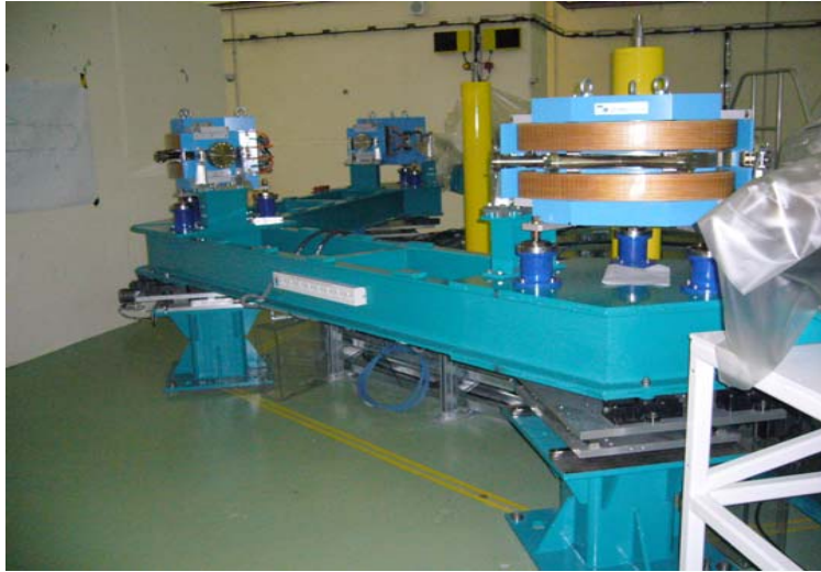
3 dipole magnets for TBA arc
