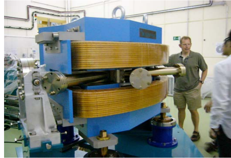
Dipole magnet with SR & alignment ports
