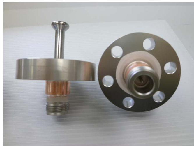
Type-II'm (i.c: Mo, o.c: Cu) "male pin"
