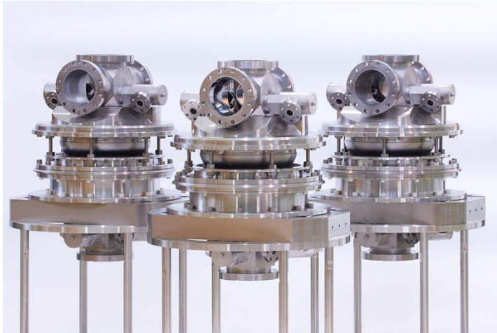
Three 2-cell Cavities
