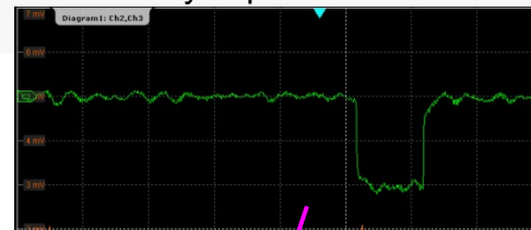
Beam-current signal at a faraday cup
