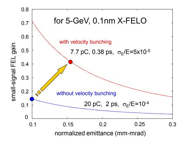
Significant enhancement of the FEL gain by velocity bunching. gain~40% is possible even with emittance growth during the bunching.
