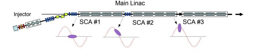
Velocity bunching in an ERL main linac was originally proposed for ultrafast X-ray pulses from undulator radiation [1].
